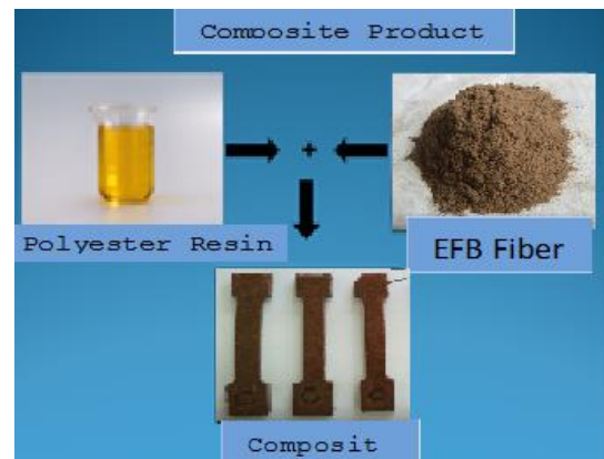
Figure 3. Composite Specimens EFB Fiber Reinforced Process.
